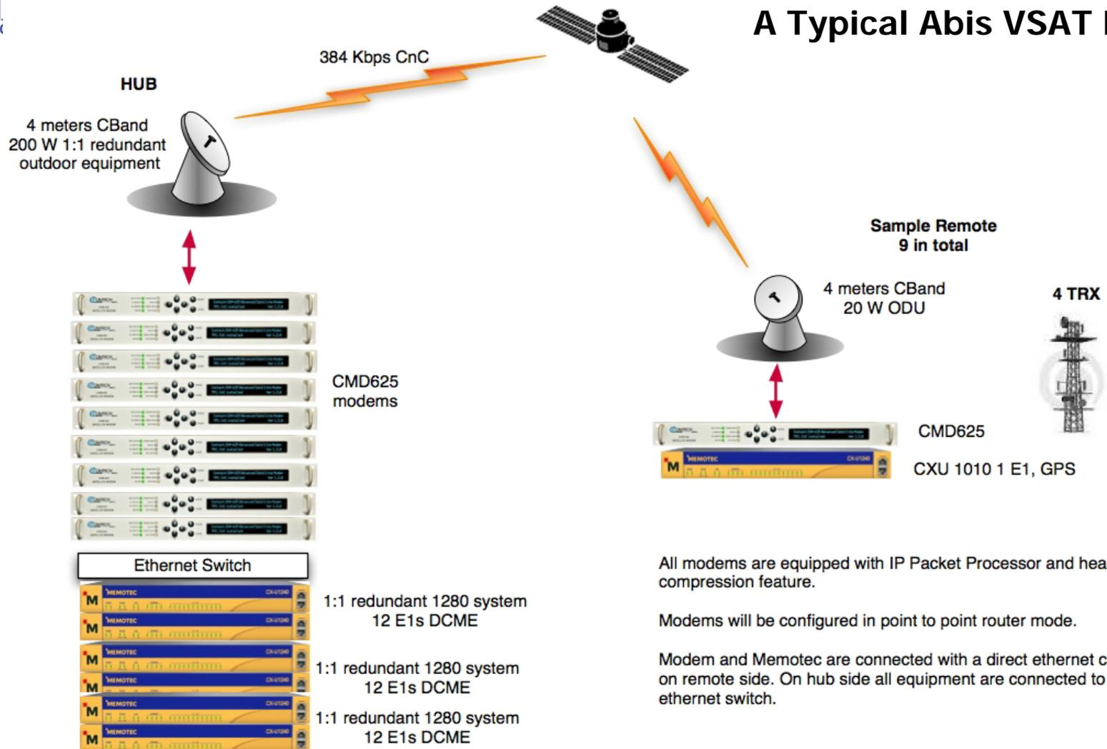
All modems are equipped with IP Packet Processor and header compression feature.
